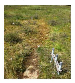
Figure 3: Hydrological studies: dip-wells and piezometers in a bog.
